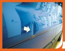
Unacceptable: Grooves, scratches and abrasions greater than 25 mm penetrating down to the base material. Deformation greater than 25 mm. Broken, cracked or bulging bumper (grille), cracked paintwork. Missing washer or tow hook covers.
